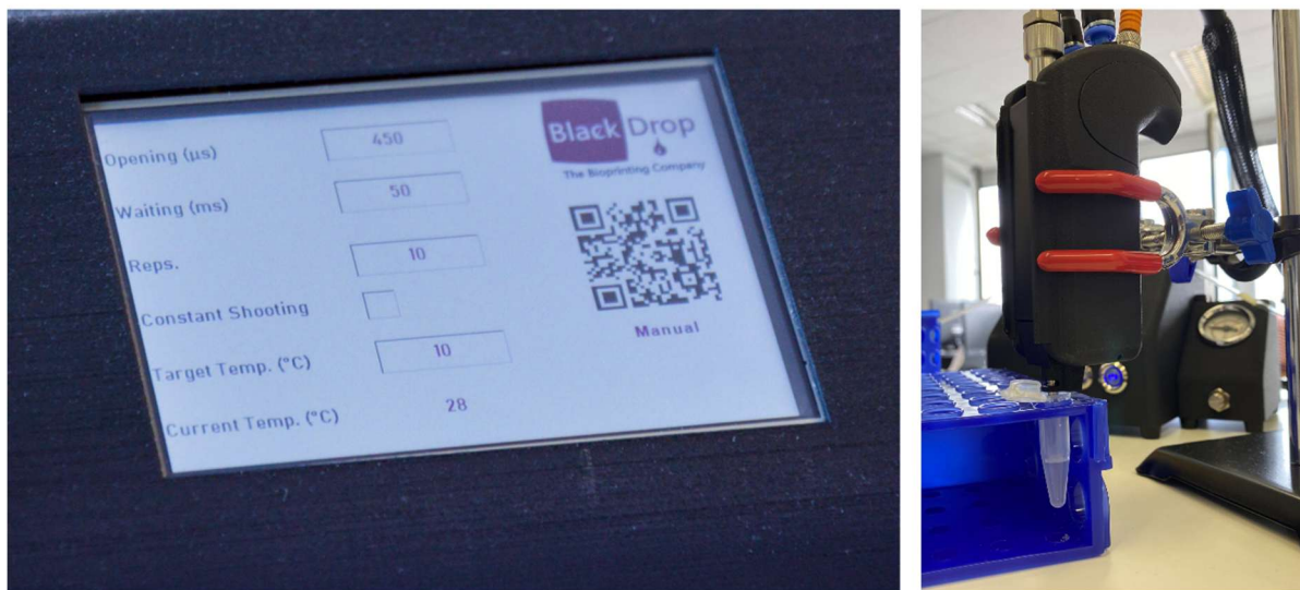
Figure 2: The touch screen (left) shows all parameters that can be controlled besides pneumatic air pressure. The DoD handheld was easily mounted in a standard laboratory stand ensuring a reproducible experimental setup (right) for dispensing alginate drops into a crosslinking solution.
