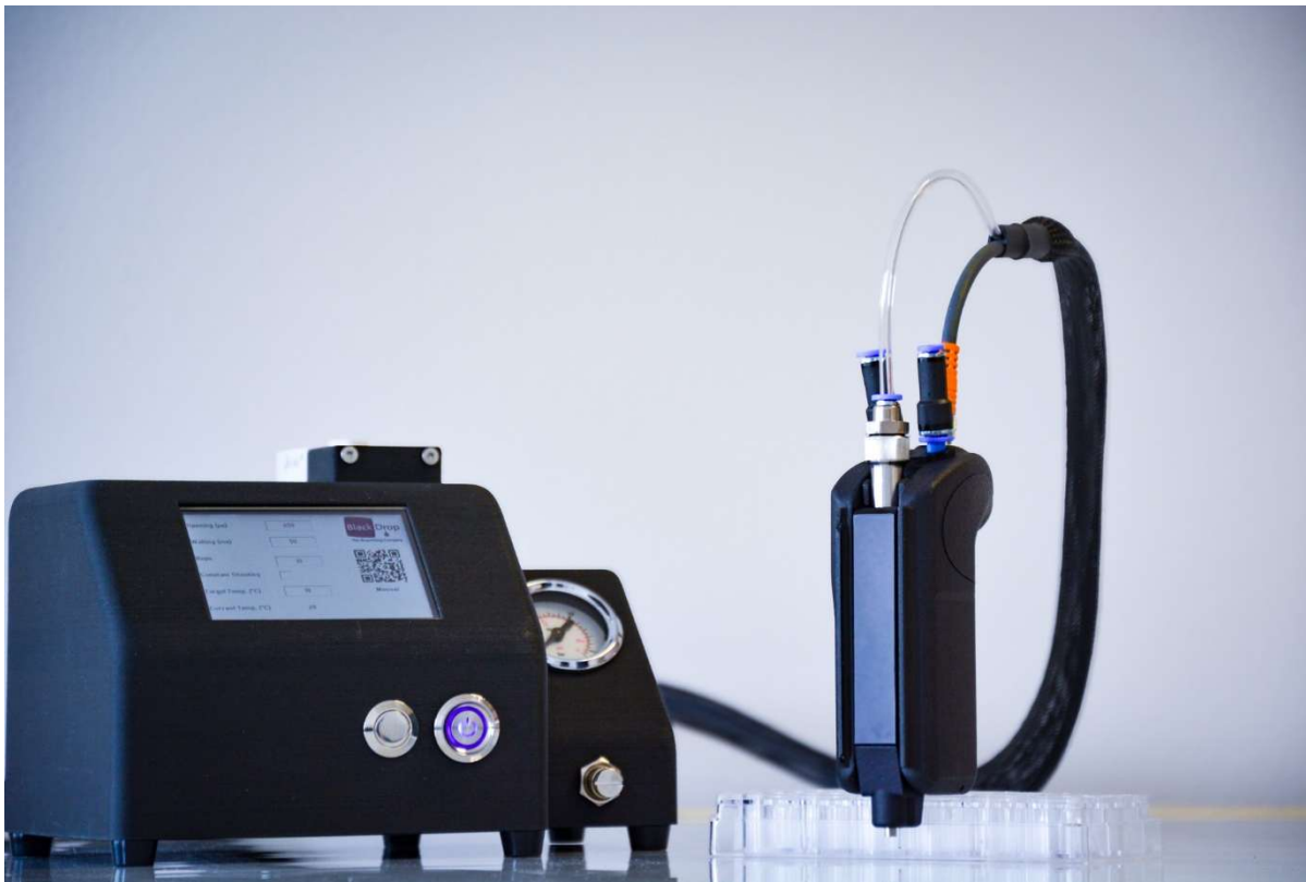
Figure 1: The Black Drop Droppgun handheld bioprinting station consists of an ergonomic handheld that allows precise bioink deposition pressing a trigger button. Dispensation parameters can be conveniently set via the touch-screen on the controlling station while the pressure of the sterile-filtered air supply can be adjusted using the manometer.
