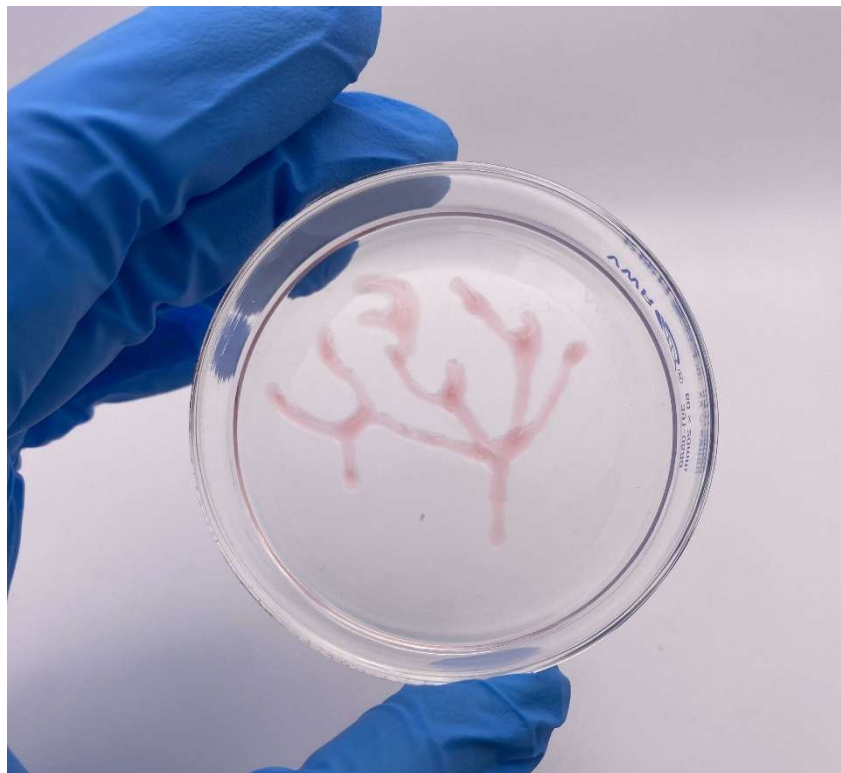
Figure 2: A biomimetic structure bioprinted using a handheld DoD printhead, illustrating the intricate details achievable with the handheld system.
