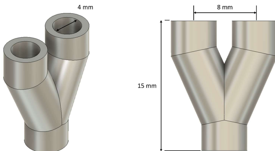
Figure 1: Dimensions of the STL file of the human sized bifurcation shown in upright position.
